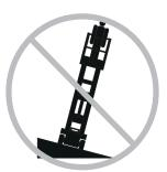
Do not depend on the tilt alarm as a level indicator. The tilt alarm sounds on the chassis and in the platform when the machine is on a slope.
