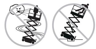
Do not drive the machine on or near uneven terrain, unstable surfaces or other hazardous conditions with the platform raised.
